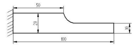
4. Loads will not be applied to the beam shown below in order to observe the deflection caused by the weight of the beam itself. The beam is to be made of steel with a Young's modulus of elasticity of 200 Gpa.
