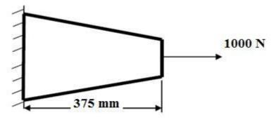
Solution: The tapered bar is modified into 2 elements as shown below with modified area of cross section.
