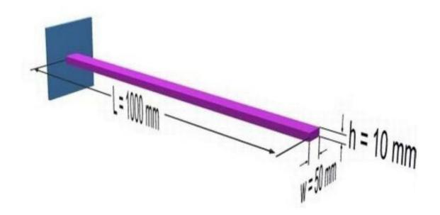
5. A beam has a force of 1000N applied as shown below. The purpose of this optimization problem is to minimize the weight of the beam without exceeding the allowable stress. It is necessary to find the cross sectional dimensions of the beam in order to minimize the weight of the beam. However, the width and height of the beam cannot be smaller than 10mm. The maximum stress anywhere in the beam cannot exceed 200 MPa. The beam is to be made of steel with a modulus of elasticity of 200 GPa
