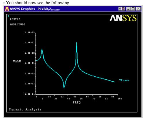
This is the response at node 2 for the cyclic load applied at this node from 0 - 100 Hz.  $\Box$  For ANSYS version lower than 7.0, the 'Variable Viewer' window is not available. Use the 'Define
